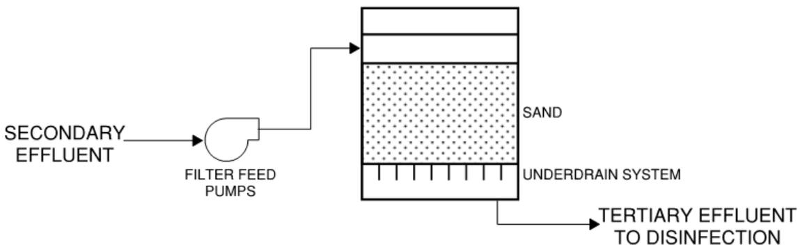
Figure 4. Alternative 2: Downflow sand filter process flow diagram. Alternative 2B is the same technology but involves 2-stages instead of single-stage filters.
