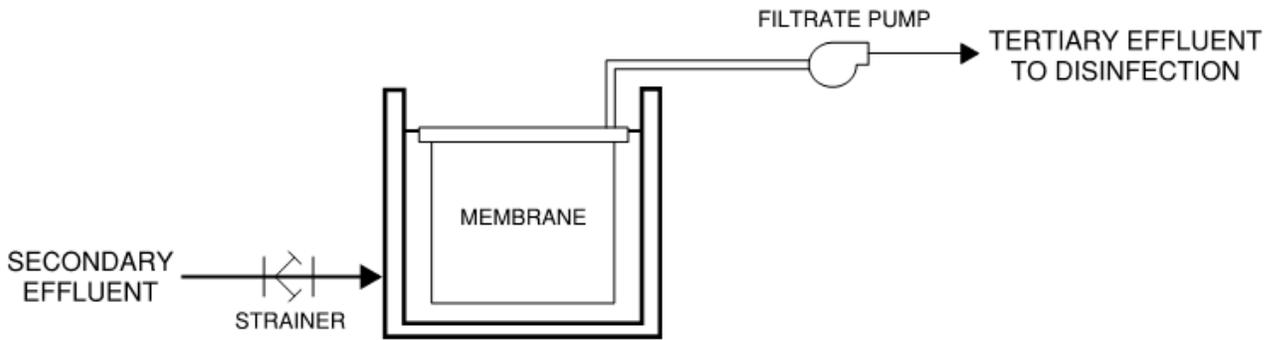
Figure 3. Alternative 1: Tertiary membrane (submerged system) process flow diagram
