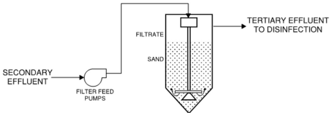
Figure 5. Alternative 3: Upflow sand filter process flow diagram. Alternative 3B is the same technology but involves 2-stages instead of single-stage filters.
