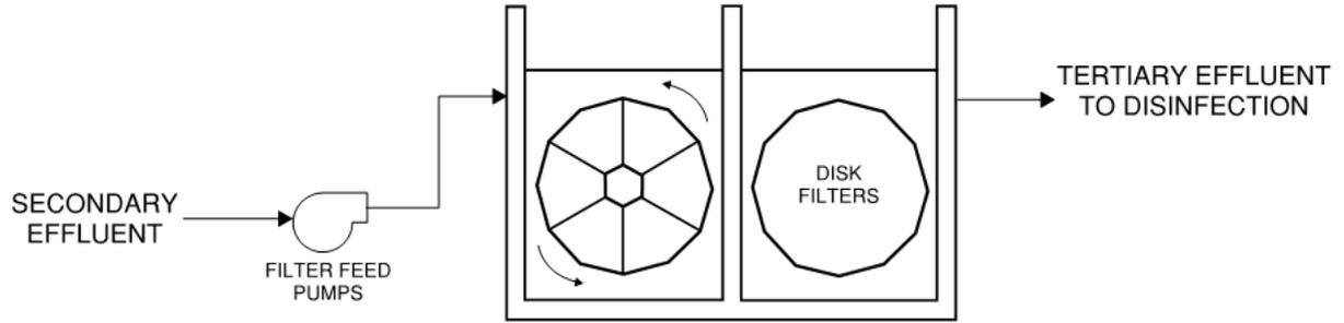
Figure 6. Alternative 4: Cloth disk filter process flow diagram
