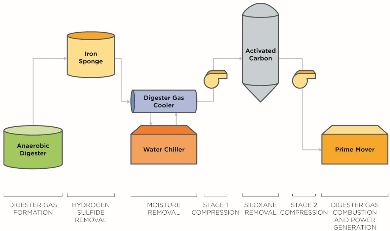
**Figure 2. Gas Conditioning System Process Flow Diagram**
