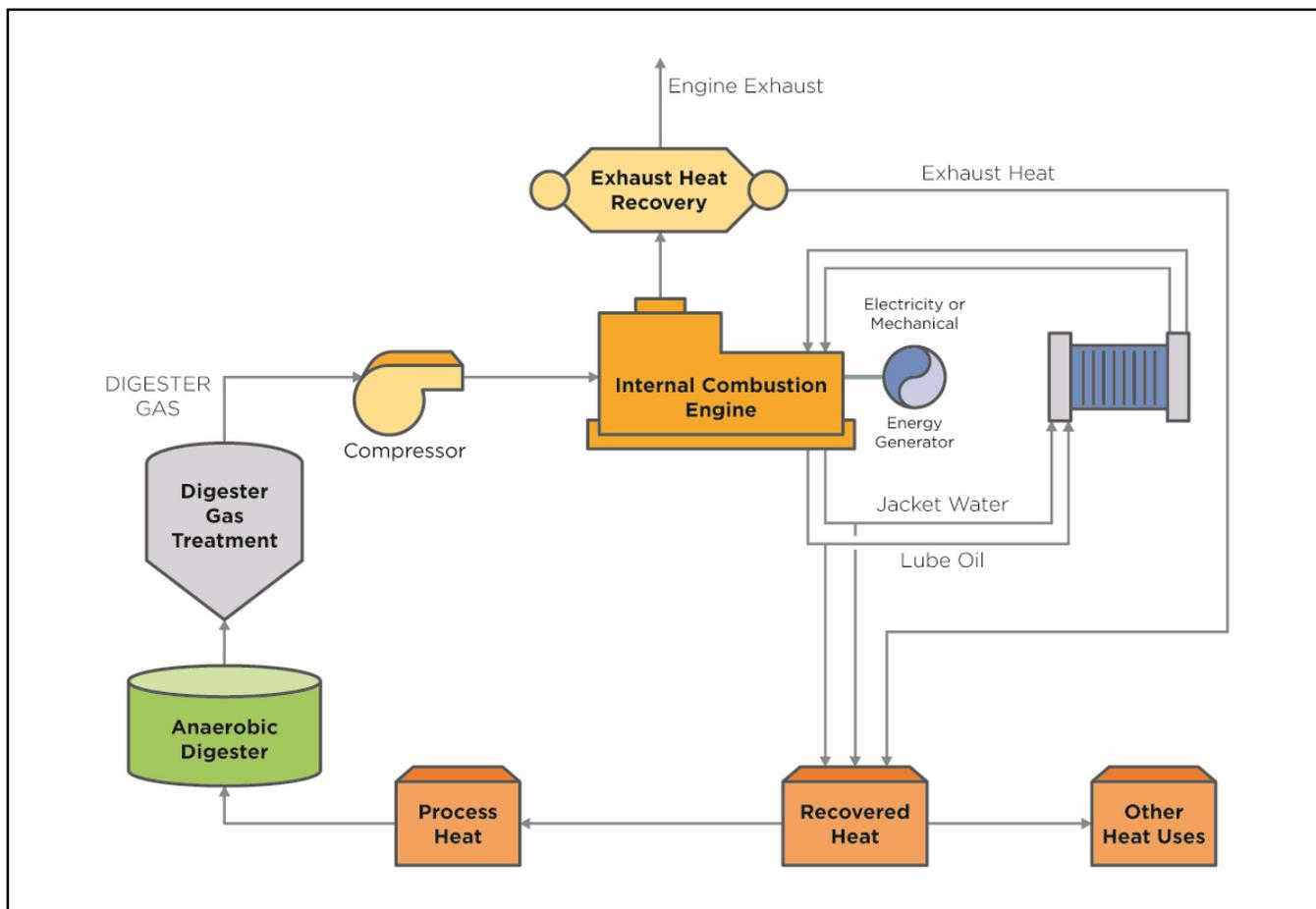
Figure 1. Cogeneration System (Alternative 1) Process Flow Diagram
