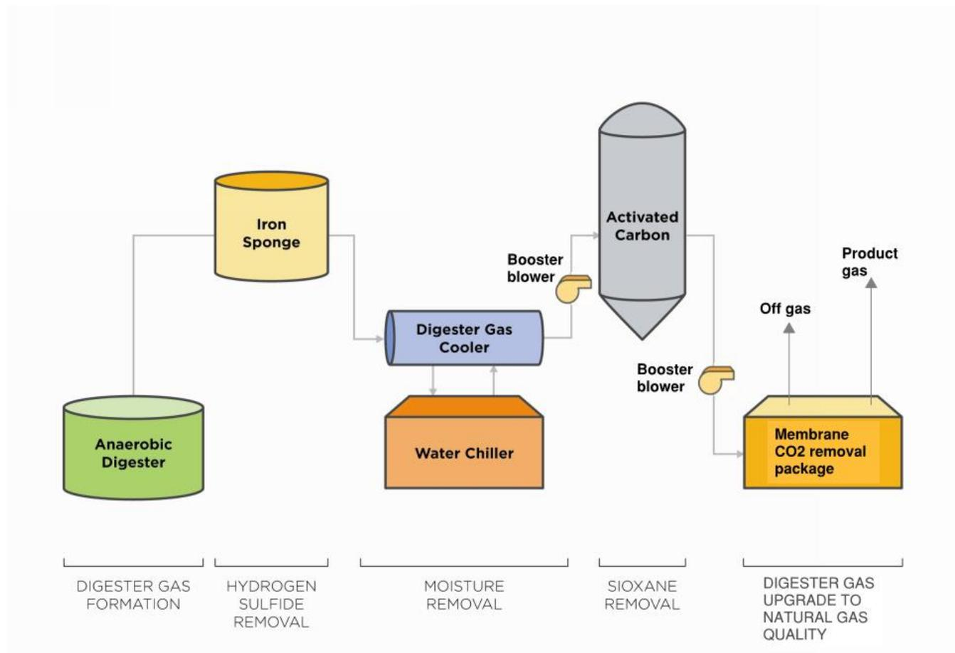
Figure 3. Renewable Natural Gas (Alternative 2) Process Flow Diagram
