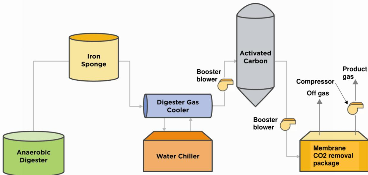
Figure 4. Compressed Natural Gas (Alternative 3) Process Flow Diagram
